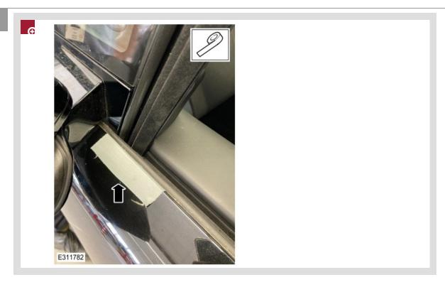
Apply a suitable masking tape to the upper area of the front door, as shown in the illustration.
