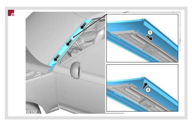
Remove the a-pillar molding by pushing with both hands and sliding down.
