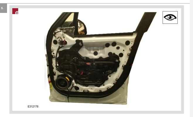
Make sure that any installed wiring harness retainers, fixings, clips, grommets and adhesive patches are all correctly installed to the door before continuing.
