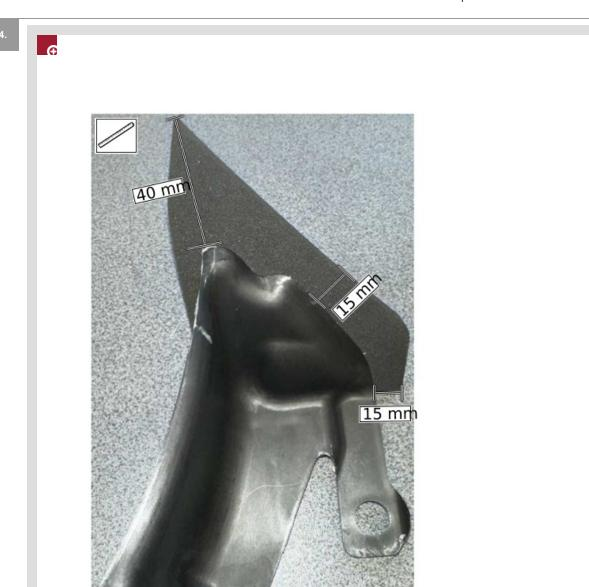
Using the measurements shown as a guide, position and hold the  $\underline{NVH}$  foam pad against the trim, as shown in the illustration.
