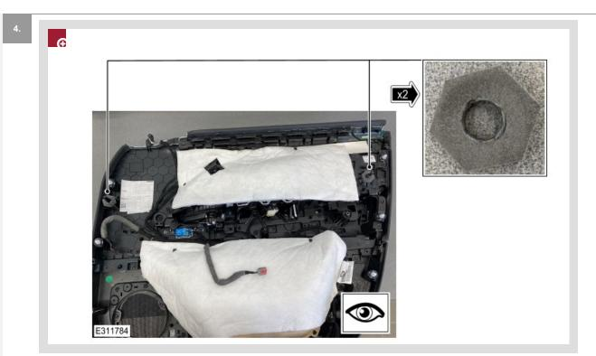
Make sure the 2 front interior door trim <u>NVH</u> pads are installed.
