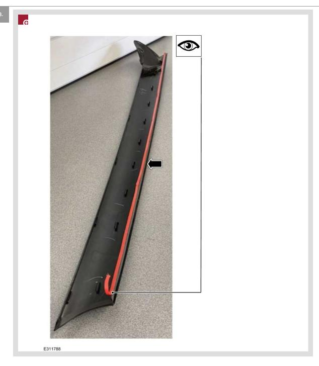
Apply 3M<sup>™</sup> Adhesive Tape - PX5011 (or an equivalent suitable double-sided tape) on top of the foam <u>NVH</u> pad. Leave a minimum of 30 mm excess backing exposed at the top of the a-pillar molding, as shown in the illustration.
