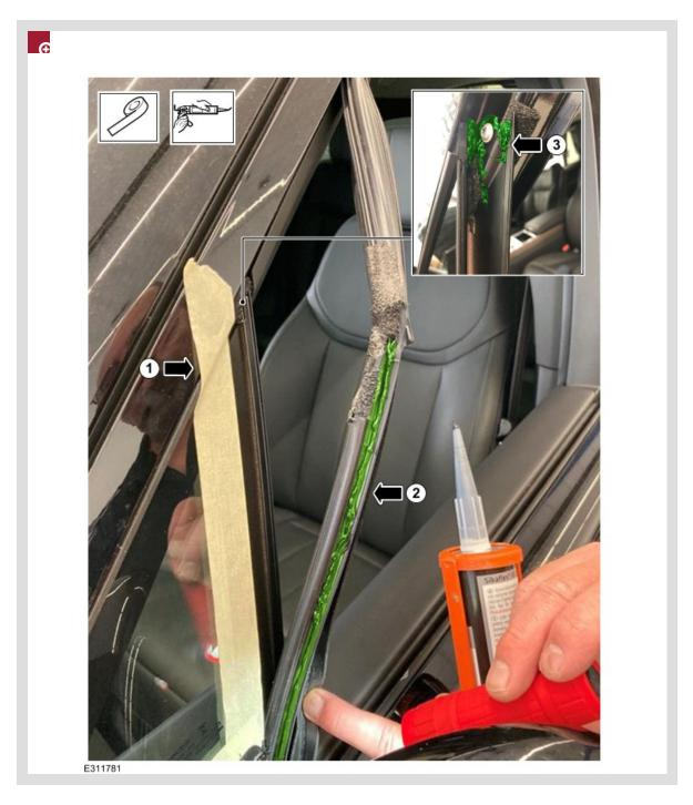
Use SikaTack OEM+ (or an equivalent suitable polyurethane glazing adhesive) to seal the front window seal.
