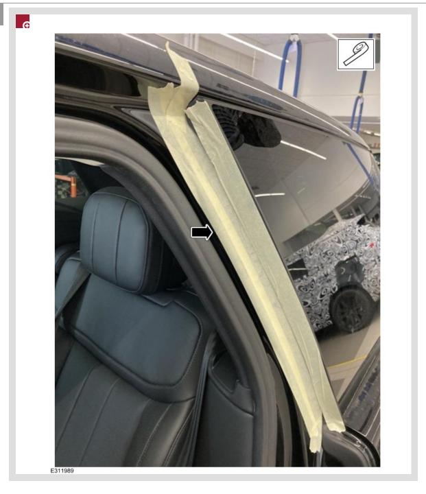
Apply a suitable masking tape to the rear quarter window seal. Make sure the window seal can still be lifted.
