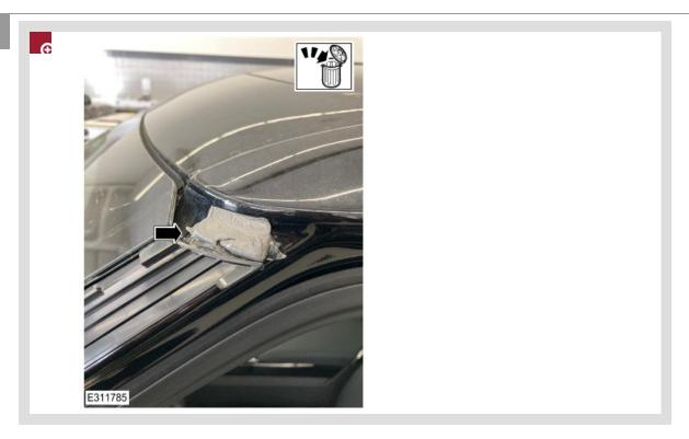
Remove and discard the  $\underline{NVH}$  pad at the top of the a-pillar.
