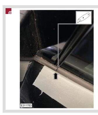
Using a suitable tool, cut through the front door outer waist seal, as shown in the illustration.
