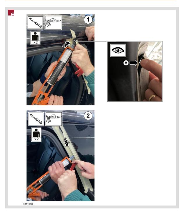
Using the aid of another technician, apply approximately 75 ml of SikaTack OEM+ (or an equivalent suitable polyurethane glazing adhesive) along the cavity behind the window seal.
