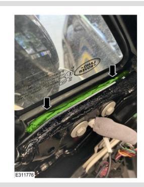
Apply 3M<sup>™</sup> Scotch-Weld 5313 (or an equivalent suitable black butyl strip) into the cavity shown. Apply enough butyl to fill the cavity without the butyl covering the top edges of the window seal and body panel.
