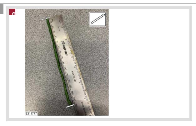
Mold a piece of 3M™ Scotch-Weld 5313 (or an equivalent suitable black butyl strip) approximately 155 mm in length and 5 mm in width.
