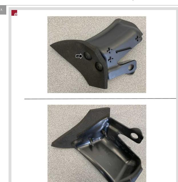
Install the  $\underline{NVH}$  pad as shown in the illustration, using the 2 holes drilled in step 6.
