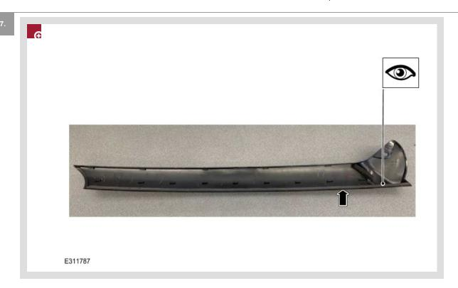
Place the a-pillar molding onto a suitable flat surface and locate the foam <u>NVH</u> pad which is applied across the length of the a-pillar molding.
