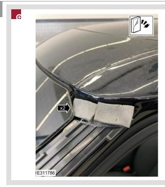
Install the new polyethylene closed-cell foam  $\underline{\mathsf{NVH}}$  pads at the top of the a-pillar.
