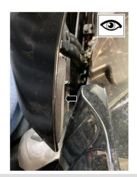
Reverse steps 2 and 3. Make sure the <u>NVH</u> pad is correctly positioned as shown in the illustration, before continuing.
