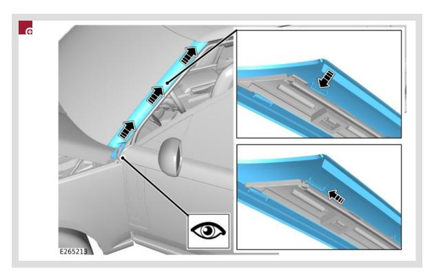
Install the a-pillar molding by pushing with both hands and sliding up.
