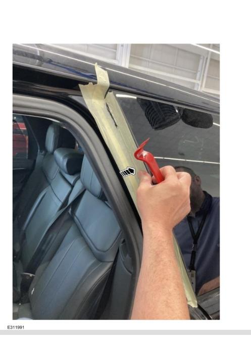
Use a finger or thumb to firm down the window seal.
