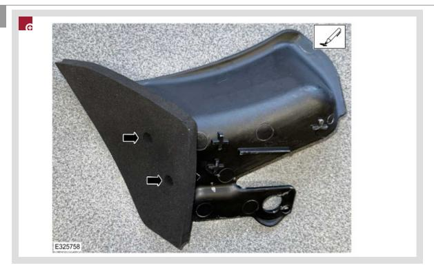
With the <u>NVH</u> foam pad still held against the trim, use a suitable marker pen to mark the trim through the 2 holes in the <u>NVH</u> foam pad.
