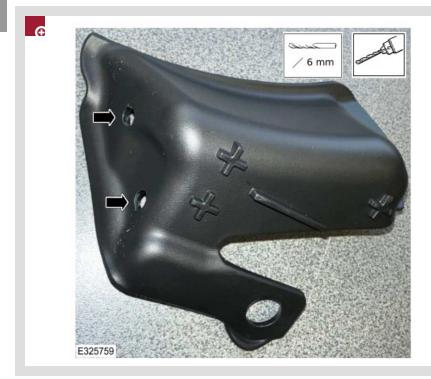
Using a suitable drill, drill a 6 mm hole through both areas marked on the trim.
