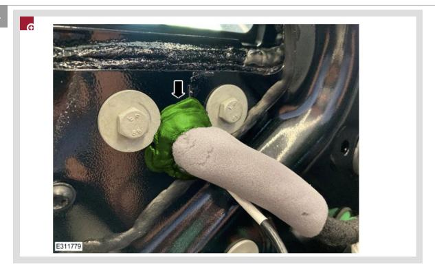
Apply 3M<sup>™</sup> Scotch-Weld 5313 (or an equivalent suitable black butyl strip) around the wiring harness, as shown in the illustration. The butyl must fully seal the hole within the body panel.
