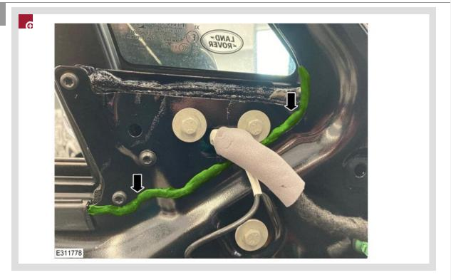
Apply the butyl along the body panel seam, as shown in the illustration.
