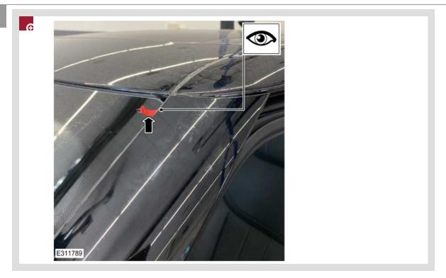
When completing step 9 below, make sure the 30 mm excess backing is positioned as shown in the illustration. This will allow the backing to be removed from the apillar molding after the a-pillar molding is installed.
