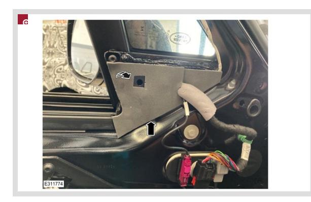
Carefully remove the adhesive <u>NVH</u> pad.
