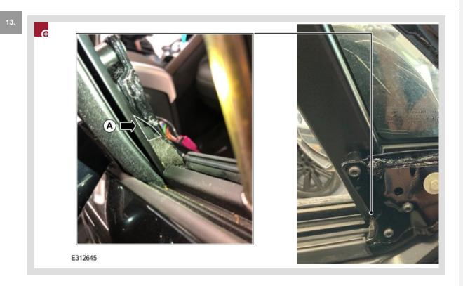
Apply 3M<sup>™</sup> Scotch-Weld 5313 (or an equivalent suitable black butyl strip) to fill the small cavity marked 'A' in the illustration, directly above the <u>NVH</u> material already applied.
