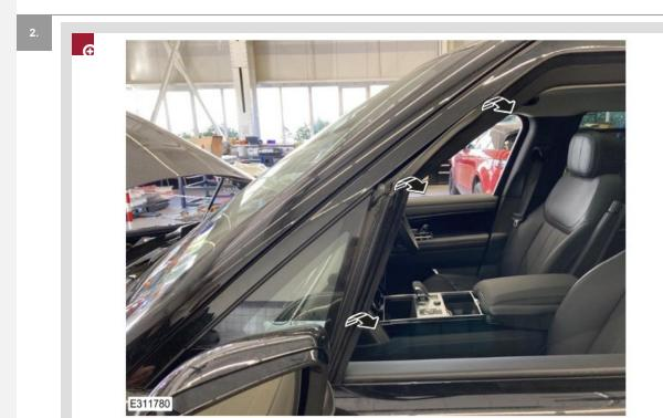
Reposition the front door window seal, as shown in the illustration.
