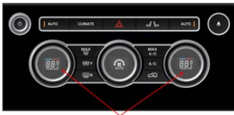
New Push function rotaries - Cabin temperature controls with new dual mode function by pushing the rotary for the heated/cooled seat feature. The rotary dial can then be adjusted to the required level (heat or cool).
