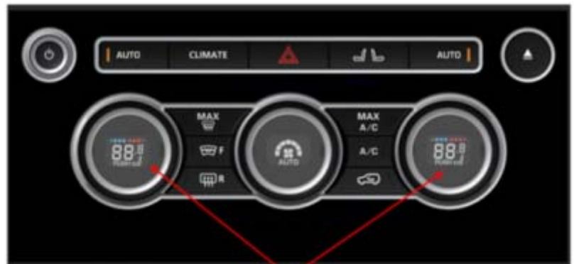
New Push function rotaries - Cabin temperature controls with new dual mode function by pushing the rotary for the heated/cooled seat feature. The rotary dial can then be adjusted to the required level (heat or cool).
