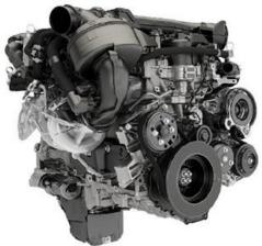
Developed from the modular design Ingenium 4 cylinder is the AJ20P6; an In-Line 6 cylinder engine equipped with a twin scroll turbocharger, Continuous Variable Valve Lift & Variable cam timing. The result is a smoother running engine that is both stronger and more efficient than the previous Supercharged V6 engines.
